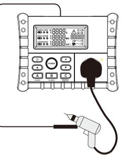
Note: The CLASS II insulation resistance test voltage is defaulted as 500VDC and can be set to 250VDC. The specific operation is shown in 6.3.
