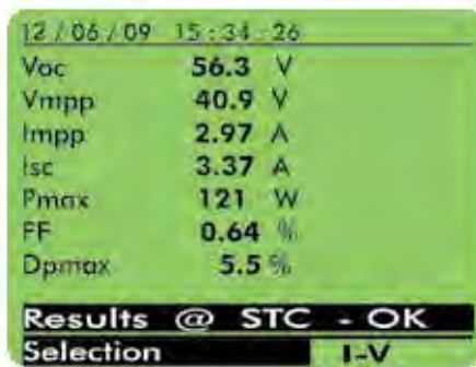
Detail of the single results of I-V Curve: OK
